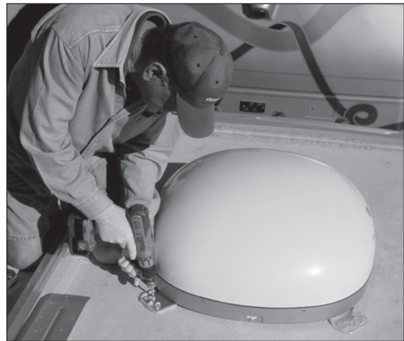
Figure 9 Attaching/Sealing the Mounting Plates
