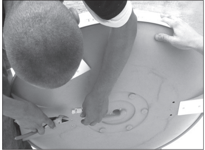
Figure 5 Removing the Shipping Restraints
